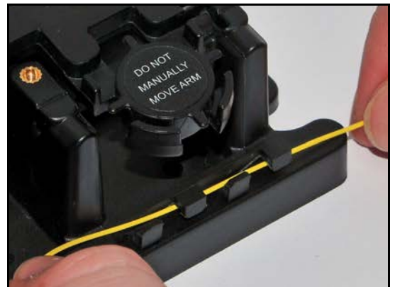
Fiber correctly routed through the lower guides
