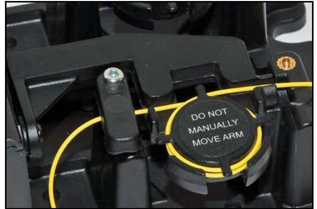
Fiber correctly routed through the guides in the paddle
