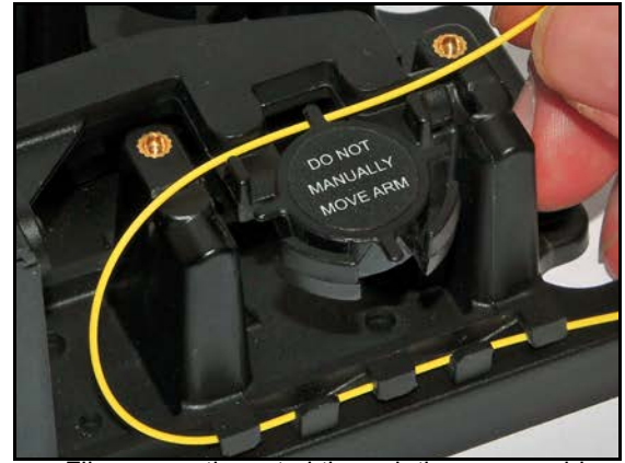
Fiber correctly routed through the upper guide
