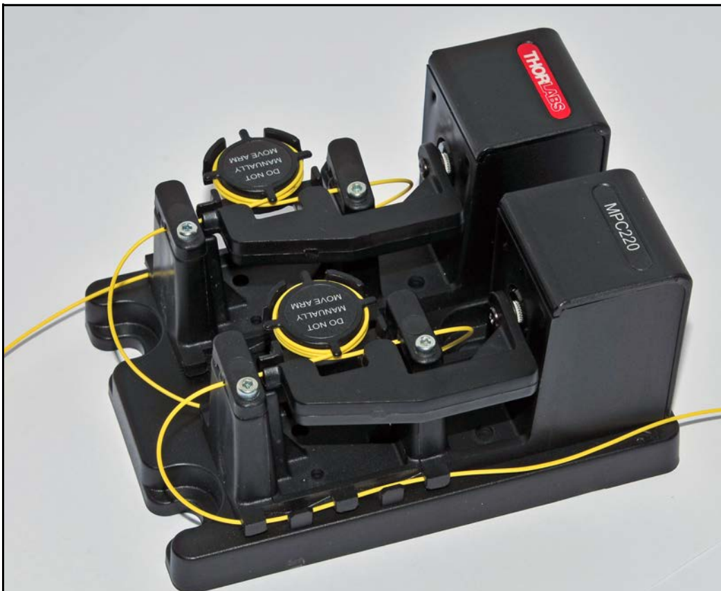
11) Working from left to right, feed the fiber into the exit guides in the base of the unit.
