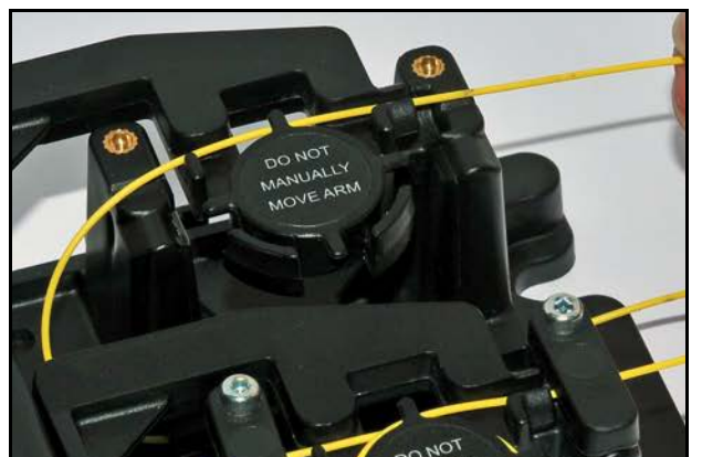
Fiber correctly routed through the upper guides on paddle 2
