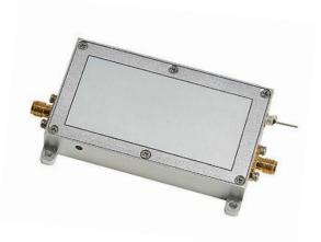
This series of AOM diver is designed for use with AOM modulator operated in an analog input control mode. This product generates heat and shall be mounted on a metal structure using fixing screws. A certain amount of space should be free around and above the product. The product is powered by + 24V DC through a per-centric capacitor.
