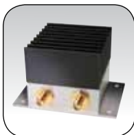
ZA2CS-2G-2W+ High Power 2 Way-0° 1.8 to 2.0 GHz P_{MAX} 20 W Unbalance 0.5°/0.05 dB
