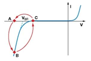
During the quenching time, which is known as the dead time of the diode, the APD is insensitive to any other incoming photons.
