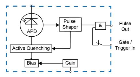
The current pulse generated by an incoming photon passes a pulse shaping circuit, which is shortening the APD's output TTL pulse duration. On the "Pulse Out" terminal the signal from the pulse shaper is applied so that counts can be viewed on an oscilloscope or registered by an external counter. In the absence of a Trigger, the gate is closed and allows signal out.
