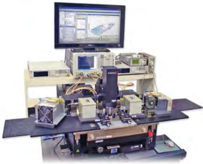
Hybrid-Active Load Pull at 30–50 GHz
